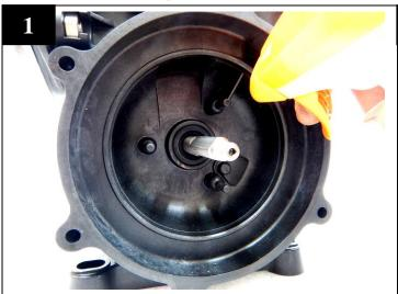
Spray water on the shaft as lubrication.
