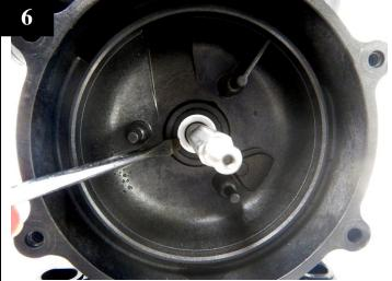
Remove ceramic parts from mech seal kit.
