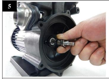
Remove the rotary parts of mechanical seal.
