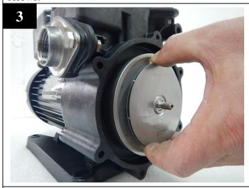
Remove all impellers, sleeves and intermediate chambers.
