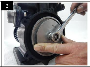
Using wrench to remove the stud bolt.
